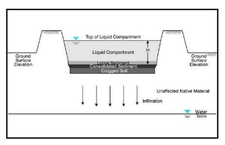
Figure 2.3 Schematic Cross-Section View of SI Unit.
